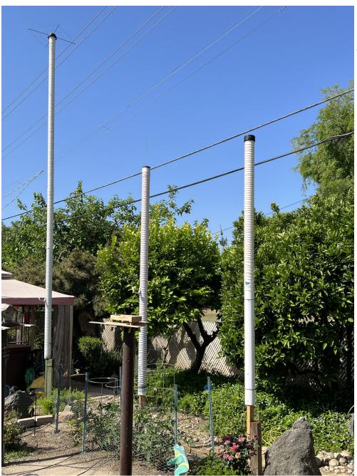
So the 40M antenna works okay. The windings start up the pole about 8ft in the air, not at near ground level like the other 2.
