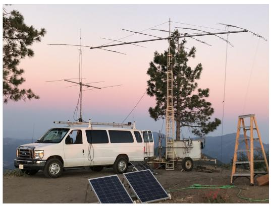
The K6MI Field Day group at 5,000 feet elevation. The M2 KT-36xa antenna is large, but needed to get the low power 5w solar powered (with batteries) signal out.
