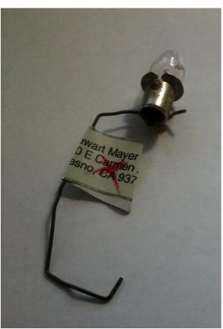
What I have done is take a #47 bulb [for your not so old kids, that was a popular bulb to use to show when your radio was on-and it is a 6.3 V bulb]; to the negative [outside] side of the bulb, I solder on a straightened paper clip with the other side bent into a U shape; the soldered wire one looks like this [the paper tab is only for use in finding the tool]:
