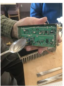
Pat, W6YEP shows the small surface mount pc board in a microwave transverter.
