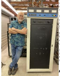
mercially available all solid state 1KW AM transmitter. It is full of lots of TO-3 transistors. It is on the air on 1925 khz, listen for it this winter.
