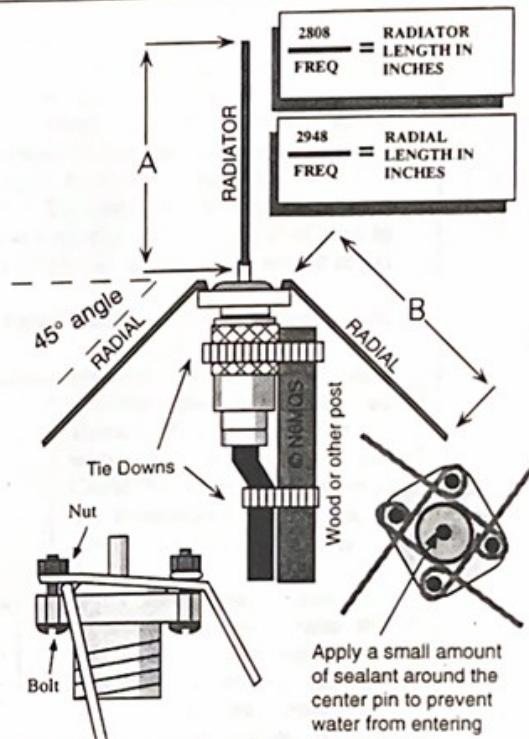
Apply a small amount of sealant around the center pin to prevent water from entering the connector
